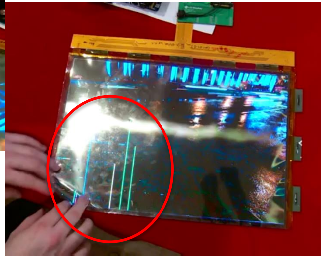
After rolling: line defects!
